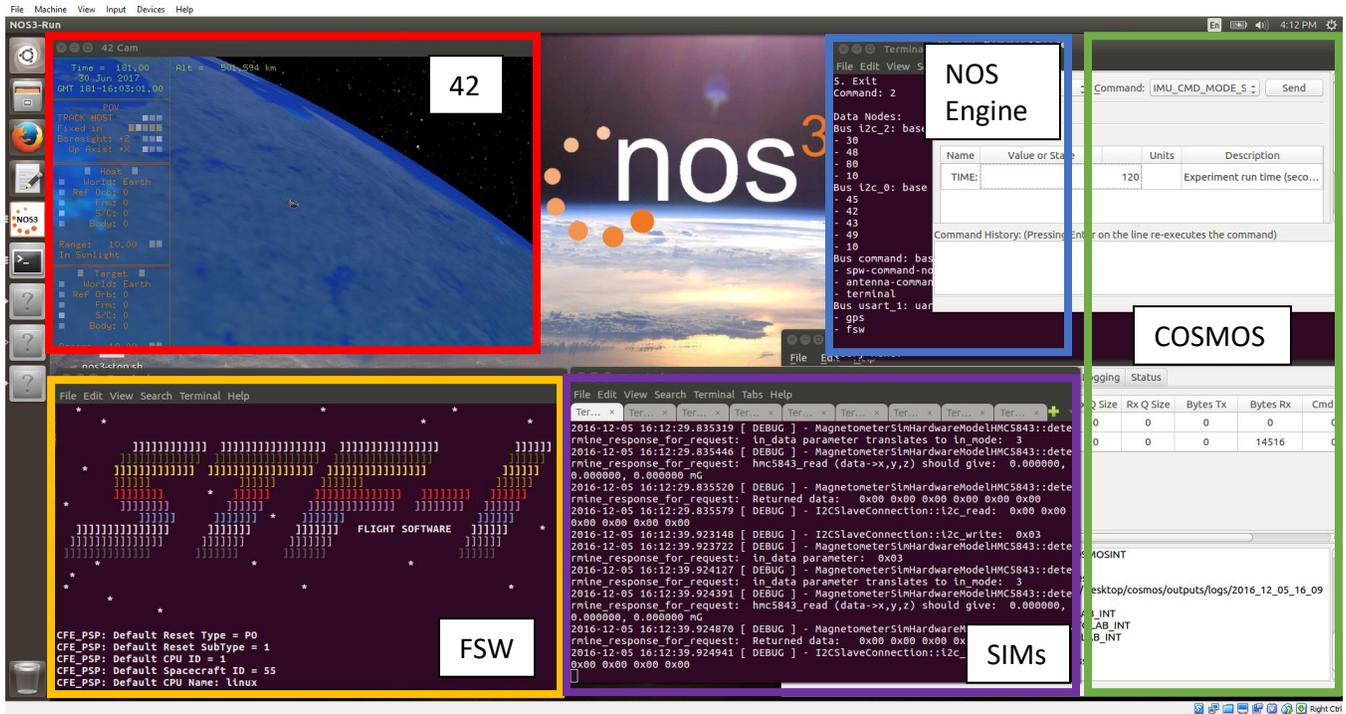
Figure 8 - NOS3 Running - Server, Simulators, 42, Flight Software, COSMOS
