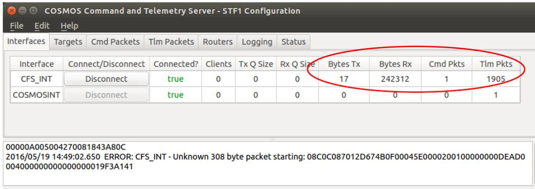
Figure 10 - COSMOS Command and Telemetry Server - Showing "Bytes Tx", "Bytes Rx"
