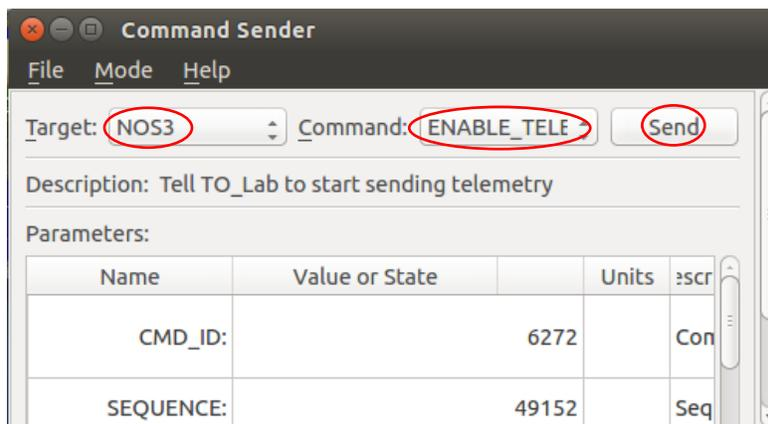
Figure 9- COSMOS Command Sending - Enabling Telemetry
