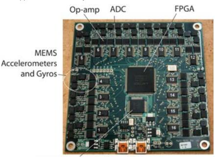
FTDI USB-serial bridge USB Figure 1 - First Generation IMU board designed for CubeSat platform
