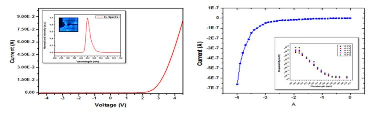
Figure 3 – (Left) Current Voltage characteristics of an LED (Right) Negative bias characteristics of a PD fabricated at WVU
