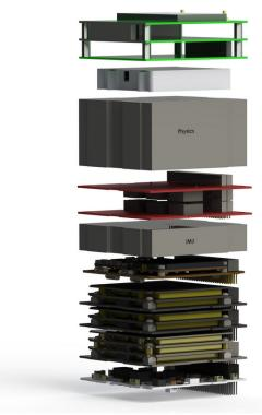
Figure 6 - STF-1 Component Stack
