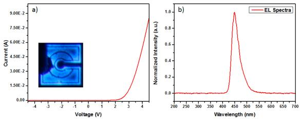
Figure 5 a) Current Voltage characteristics (Inset: Optical Image of LED) b) Electroluminescence spectra with a peak at 460 nm
